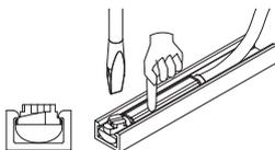
Keep the sensor in its position and screw the fastening plate to fix the sensor in the groove.
