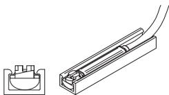
Check the correct position of the sensor in the groove. Turn it to the wished position for detection.
