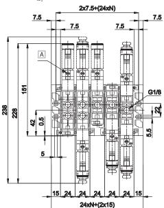
When assembling the manifold put the sub-base on a flat surface and tighten the special screw supplied. This will give perfect alignment.
